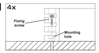
Then uphold the amplifier to the chosen position and fix the screws through the mounting holes into the drilled screw holes.
